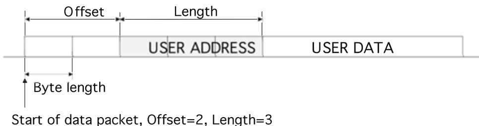
A transmitting radio modem adds a routing header and a tail to the user message. Consequently, a radio modem that receives the message removes the header and tail - so the Message Routing scheme is transparent to the user protocol.
