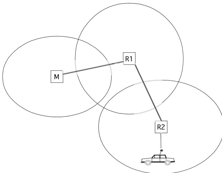
The over hop function allows for the use of mobile substations. In the example above, a mobile substation is first located in the coverage area of repeater R2. The route is defined as M, R1, R2 and vehicle. When the vehicle moves to the coverage area of repeater R1, the radio modem
