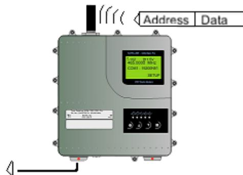
Reception addressing has been set ON, but both the primary and secondary RX addresses of the radio modem are different from the address of the received data packet.
