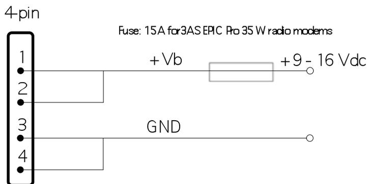
NOTE! In Epic Pro 35W the voltage is limited to 16V.
