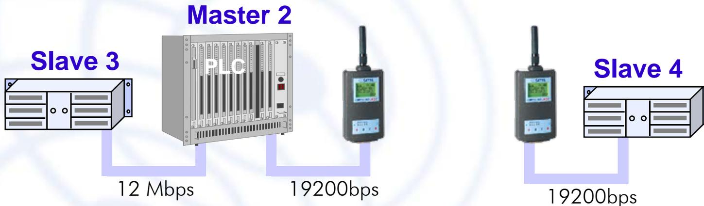
System with two bus segments. The master has a separate interface card for radio modems. The wireline system can run at the full speed.
