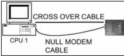
*PC connected to IP-LINK with Ethernet crossover cable for data transfer.*
