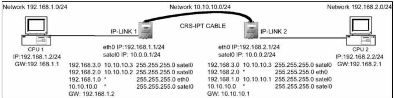
IP-LINKs connected with test cable CRS-IPT.
